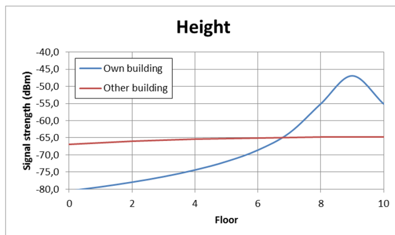
Figure 25 Received signal strength versus height (floor) indoor Wi-Fi system and drone inspecting 9 th floor
