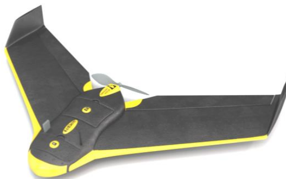
Figure 5. Example of a fixed wing drone, the SenseFly eBee, mostly used for mapping
