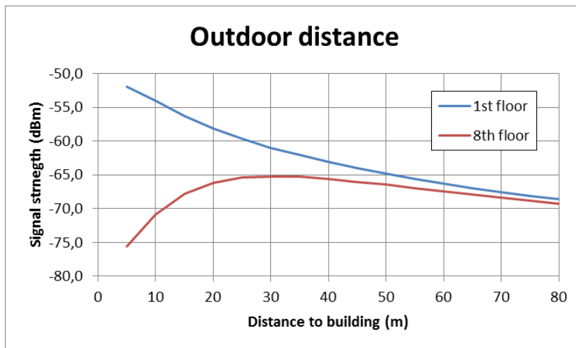
Figure 24 Received signal strength versus outdoor distance to building for 1 st and 8 th floor
