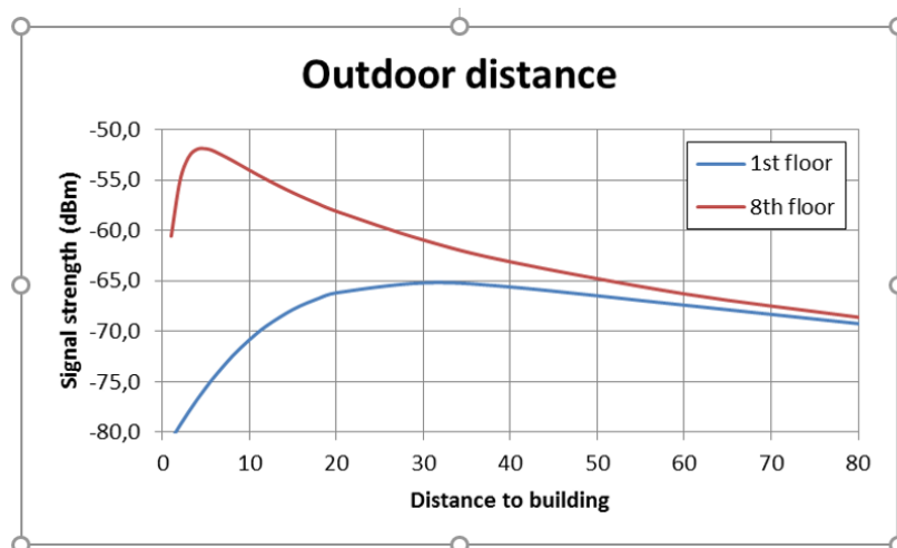
Figure 27 Received signal strength versus outdoor distance to building for 1 st and 8 th floor
