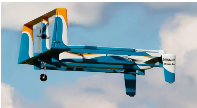
Figure 6. Example of a hybrid VTOL drone, the Amazon Prime Air
